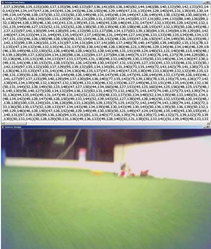
Fig. 2 Raw image data represented as a string of triples, as processed by a robot’s vision processing system ( top ), and the corresponding data represented as an RGB image for humans to understand ( bottom )
