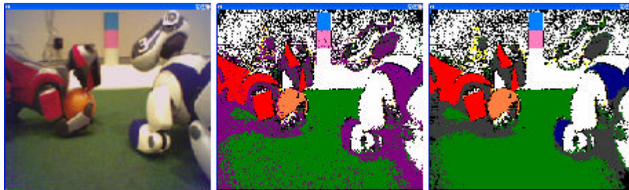
Fig. 1. An image from an AIBO ERS7 ( left ), the overlapping colors in the corresponding image are represented in purple ( centre ), and the processed image in which overlapping colors are assigned to symbolic colors ( right ). In the raw image there is a blue discoloration around the edge of the image, and there is little contrast or separation between the robot's blue uniform, shadows on the field, and the darker colors of each robot. The blue uniform consists almost entirely of maybe-colors.
